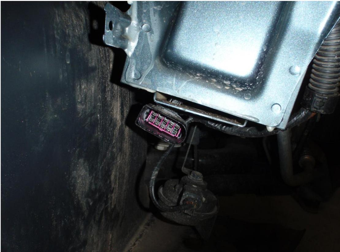
On the right side of the vehicle, unplug the connector from behind the headlight, and remove the clip securing the wiring to the chassis, then push the plug backwards in the direction of the wiring to remove it from behind the headlight.
