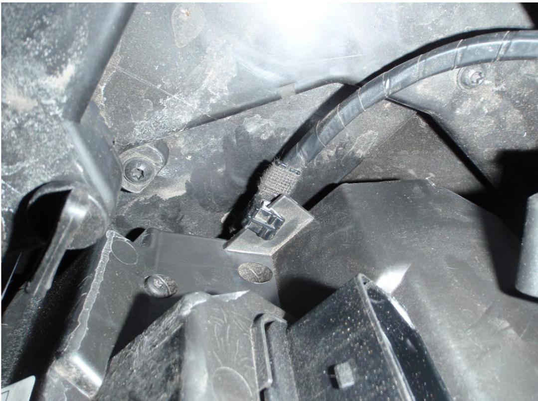
11. Finally remove the last two T30 screws behind the central moulding to release the bumper, and remove it from the car.
