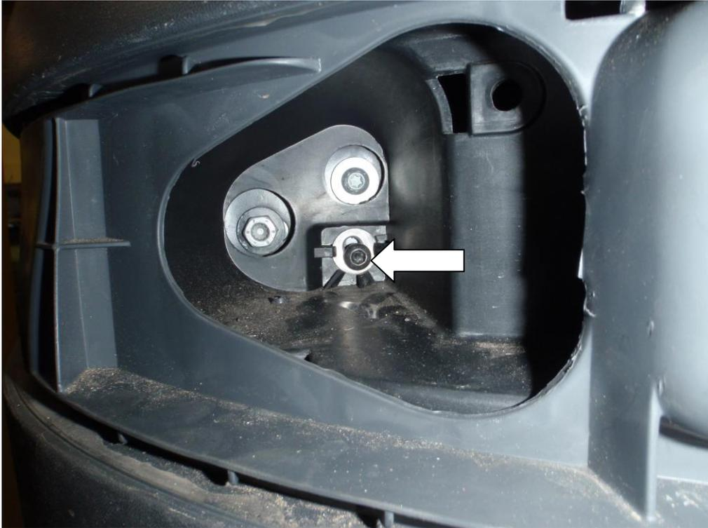
10. The electrics that pass through the bumper will need to be unplugged (our model has no foglights so these will need to be removed also). On the left side of the vehicle (from the front) undo the electrical connector inside the inner arch, just inside the arch liner.
