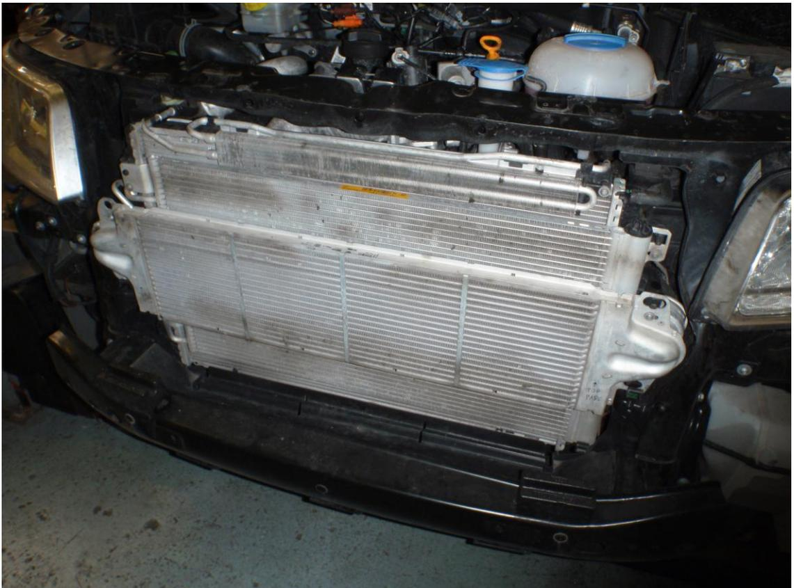
12. Remove the two T30 screws securing the intercooler to the chassis
