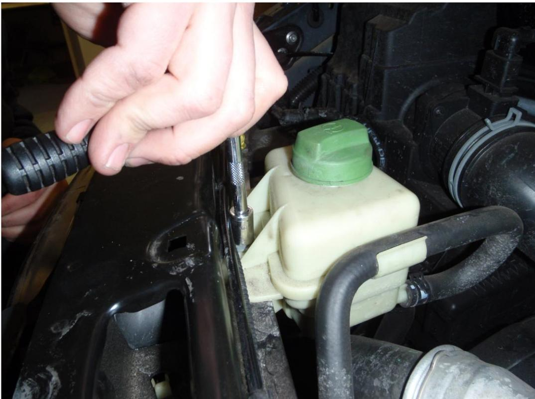
5. Behind the power steering reservoir, you can now see the single T25 screw that needs to be removed, and in the hole underneath it, another T25 screw. Repeat for both sides of the vehicle.
