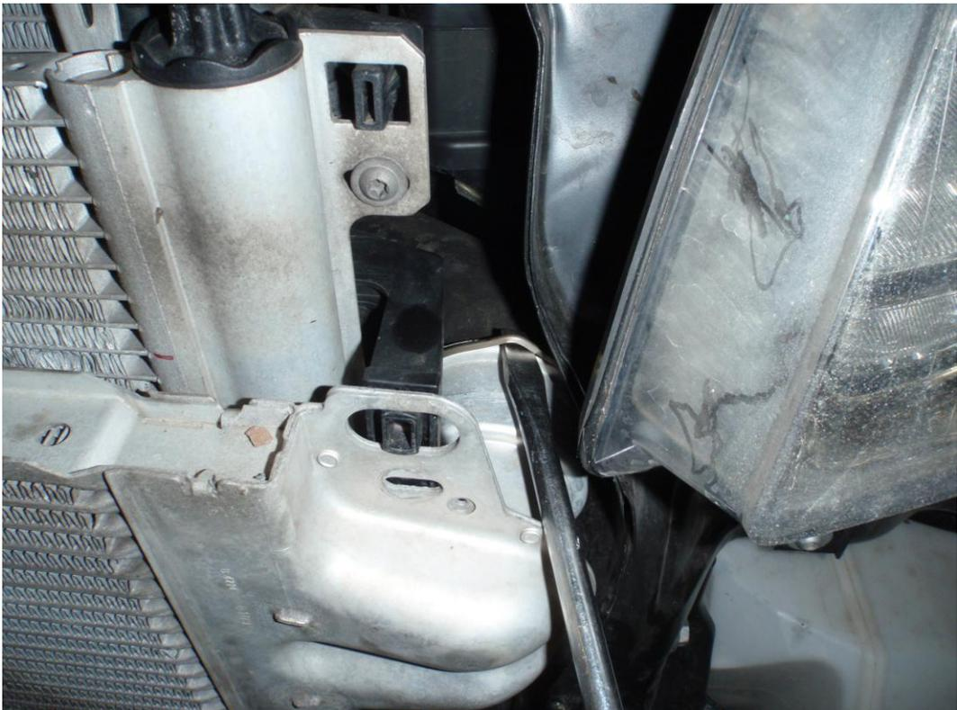
14. Remove the hose retaining clips from the stock intercooler and place them on the Forge intercooler in the same orientation. Place the Forge core on the vehicle and push the hoses in until they click into the retaining clips. Reuse the T30 screws to attach the Forge core .
