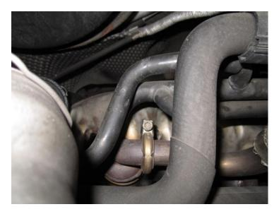
3. Using the OEM clamp you have just removed, fit the Forge Motorsport blanking plate and tighten the clamp using a 6mm Allen key .The Forge Motorsport blanking plate is pictured below.
