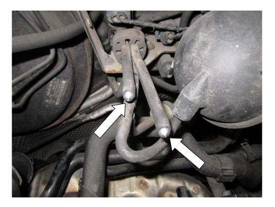
8. Remove the OEM O-ring from the male coupler on the boost pipe you removed in section 4 and place into the supplied Forge Motorsport coupler.
