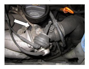
2. Once the 13mm bolts have been removed using a 6mm Allen key remove the clamp that holds the other end of the exhaust breather in place.
