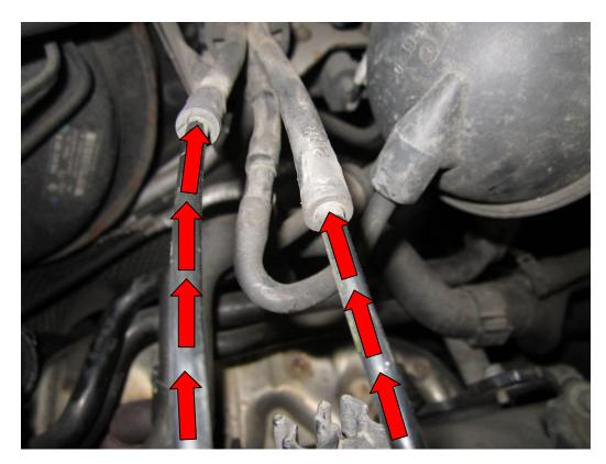
7. Place the vacuum blanks in place of the two hoses you have just disconnected as pictured below.
