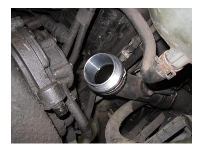
10. Fit the new O-ring supplied into the groove of the new EGR delete and then fit into the position of the EGR housing removed in section 5.
